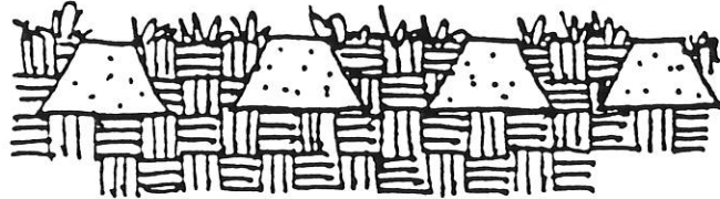
Grass block paving allows traffic movement and also the inflow of water into the soil
