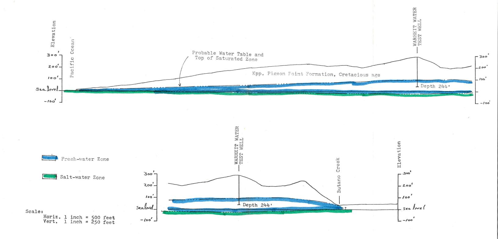
FIGURE 3, -- TOPOGRAPHIC AND HYDROLOGIC SECTION ALONG A LINE DRAWN THROUGH THE WARHEIT WATER TEST WELL FROM THE PACIFIC OCEAN TO BUTANO CREEK NEAR PESCADERO, CALIFORNIA
