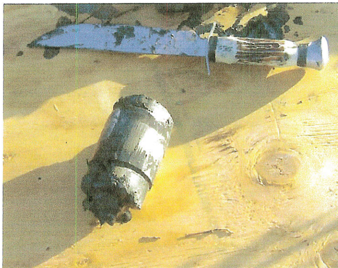
Figure 3. Intact soil core extracted from well-casing 8.
