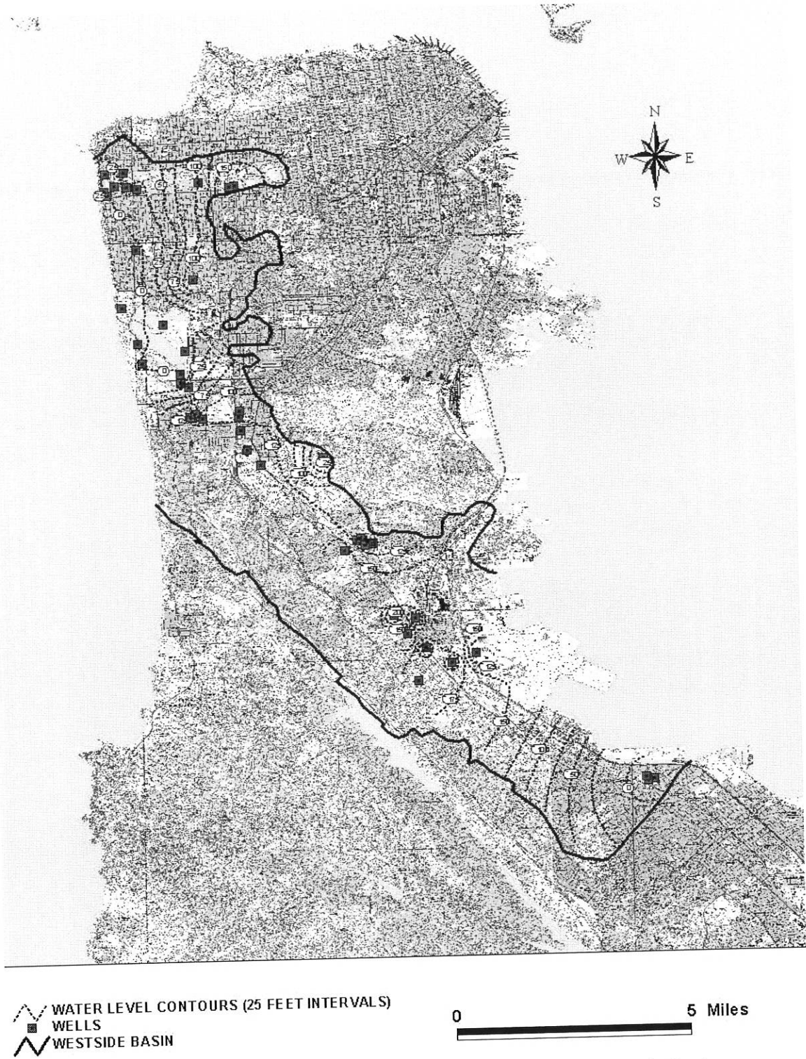
Figure 3.3: Water level conditions for the deeper aquifers of the Westside Basin on 10/25/01 after a 6-hour well shutdown. Source: San Mateo County Environmental Health Division (2002b).
