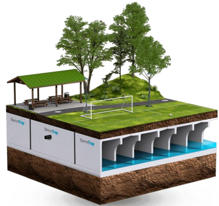
Figure 1.15. Subsurface storage system, generic example. ( http://stormtrap.com/products/singletrap/ )
