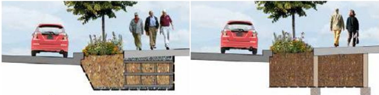
Figure 1.9. Stormwater tree well filter conceptual examples: modular suspended pavement system (left), column suspended pavement system (right).
